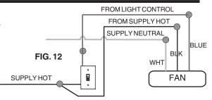
Now tuck the wires and wirenuts carefully into outlet box. Make sure the Green and White wires are tucked into one side of the box and the Black and Blue wires are tucked into the other side of the box. Make sure wirenuts remain tightly on connections.
